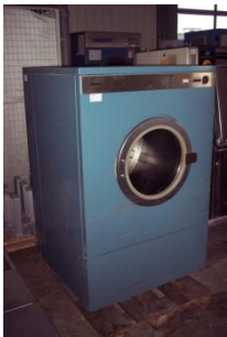
ID6859 Dryer Miele T5248, year : 1985 charge : 19 kg / 480 l, electric
