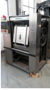
ID7011 Washer extractor Lavatec LX308, year : 1998 charge : 36 kg, steam-heated, 2-splitted drum, Medicare
